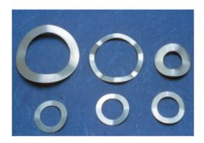
The number of waves can be two, three or more. The spring rate is proportional to the number of waves raised to the fourth power. Wave Washers are generally preferred as cushion spacers between parts on shafts or to take up the probable deviation in assembled parts. These are positioned underneath a nut, an axle bearing or a joint to reduce friction, avoid leakage, isolate, stop loosening or distribute pressure. IIS has ready stock of all the sizes. For details checkout our website.
